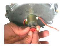
\*The primer may need to be adjusted so the engine starts easily. By holding the wahser behind the red adjusting knob, turn the adjusting knob counter-clockwise for less fuel and clockwise for more fuel.
