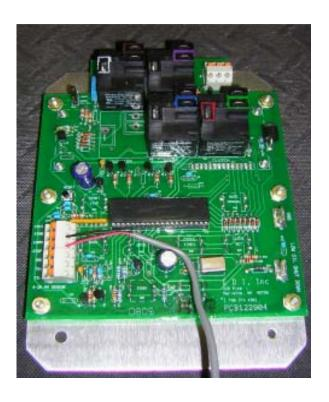
When external inputs (example: low compressor oil pressure switch) are connected to the terminal strip located at the upper right corner on the back of the board, connecting to the middle terminal (common) and either side of the terminal block, the external inputs will cause the following action:
