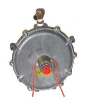
\*The KN-Regulator is used to supply gas to the engine. The Electric Primer engages when the ingnition is turned on to start the engine and disengages after the engine starts. (Only engaged when the starter is running.)
