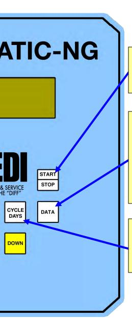
**Start/Stop:** Press the Start/Stop button to manually start and stop the motor. In automatic mode, press the Start/Stop button to stop the motor.
